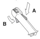
Make sure the throttle control is locked at the idle setting when the throttle lockout is released.
